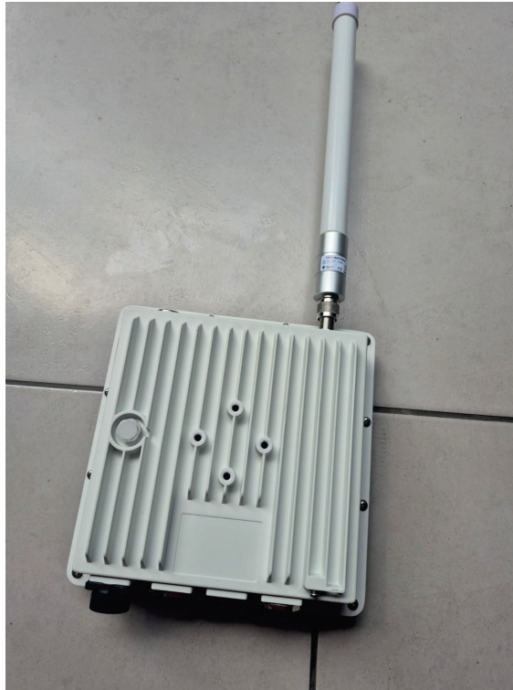
Figure 9 – Wisgate Edge Pro gateway with 3.0 dBi omnidirectional antenna.
